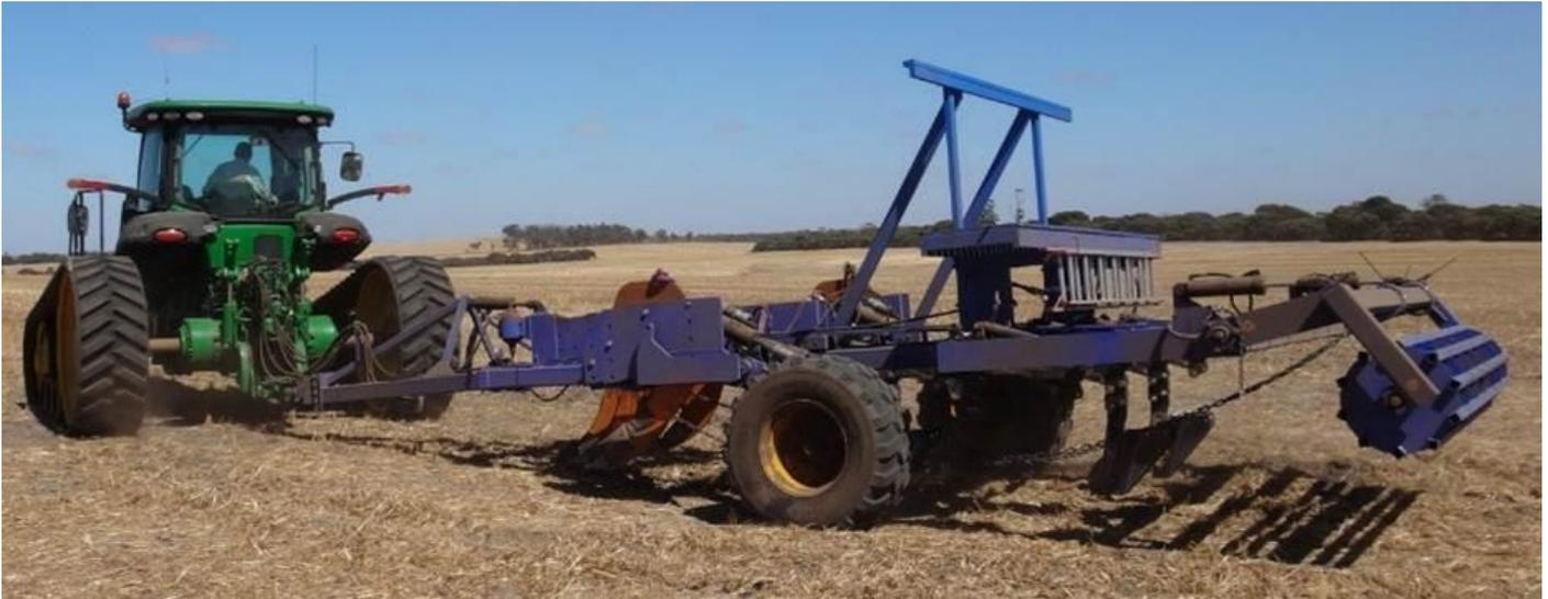
Photo 1: DAFWA's research ripper with shallow leading parabolic tines set at an aggressive angle. The front tines work at 300mm and the back tines work to 600mm. Topsoil slotting plates are attached to the back tines that run at the base of the topsoil (about 100mm). The Grizzly hydraulic crumbler roller levels, creates a firmer seed bed and crushes some clods.
