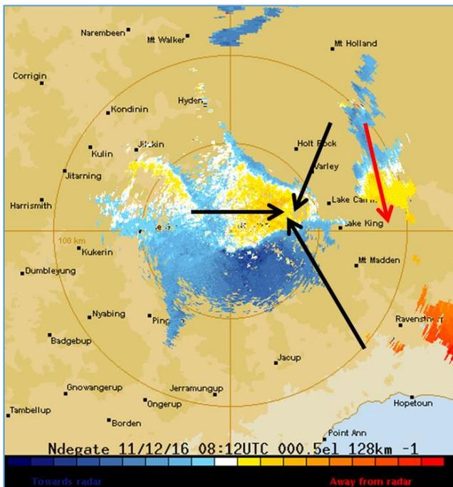
Fig 4. Display of wind components and resulting wind vectors from the Newdegate Doppler radar.
