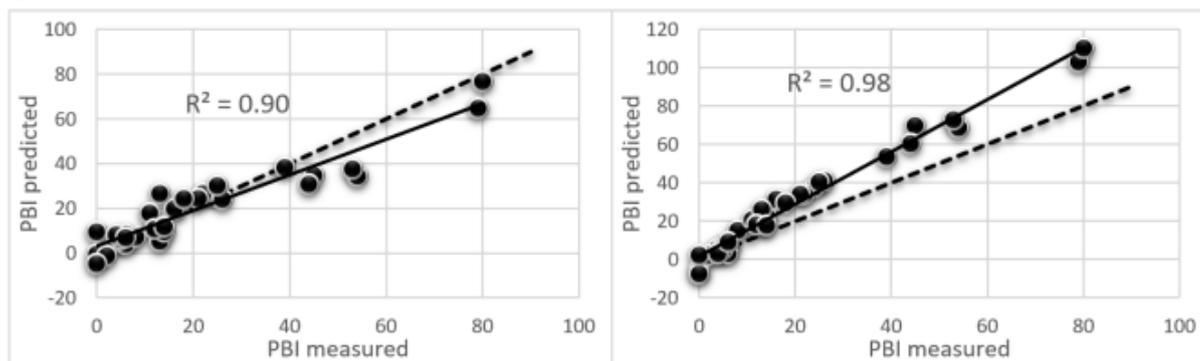
**Figure 1.** Site-specific validation of PBI values from Exoscan spectra of field-moist Karoonda soils versus laboratory determined PBI. PLSR calibration models derived from only PBI data and MIR spectra (left), and PBI data and MIR spectra plus soil moisture contents (right).
