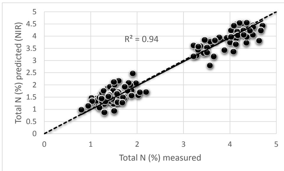
Figure 2. Cross validation of measured total N crop values with predicted crop N contents using portable NIR in field spectrometer.
