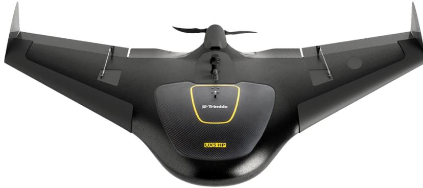
This drone can carry a full frame sensor (35mm lens) 36 megapixel mirrorless SLR camera – Sony alpha 7r. Fitted with a high quality lens, this drone is capable of capturing 1cm pixel resolution images from 80m altitude while travelling at 90 kph. The great news is that Peter Chaplyn from Quantum purchased this drone at a cost of \$80K. Not only does it capture great images, it has 5cm accuracy geo-referencing capability when used with a base station.
