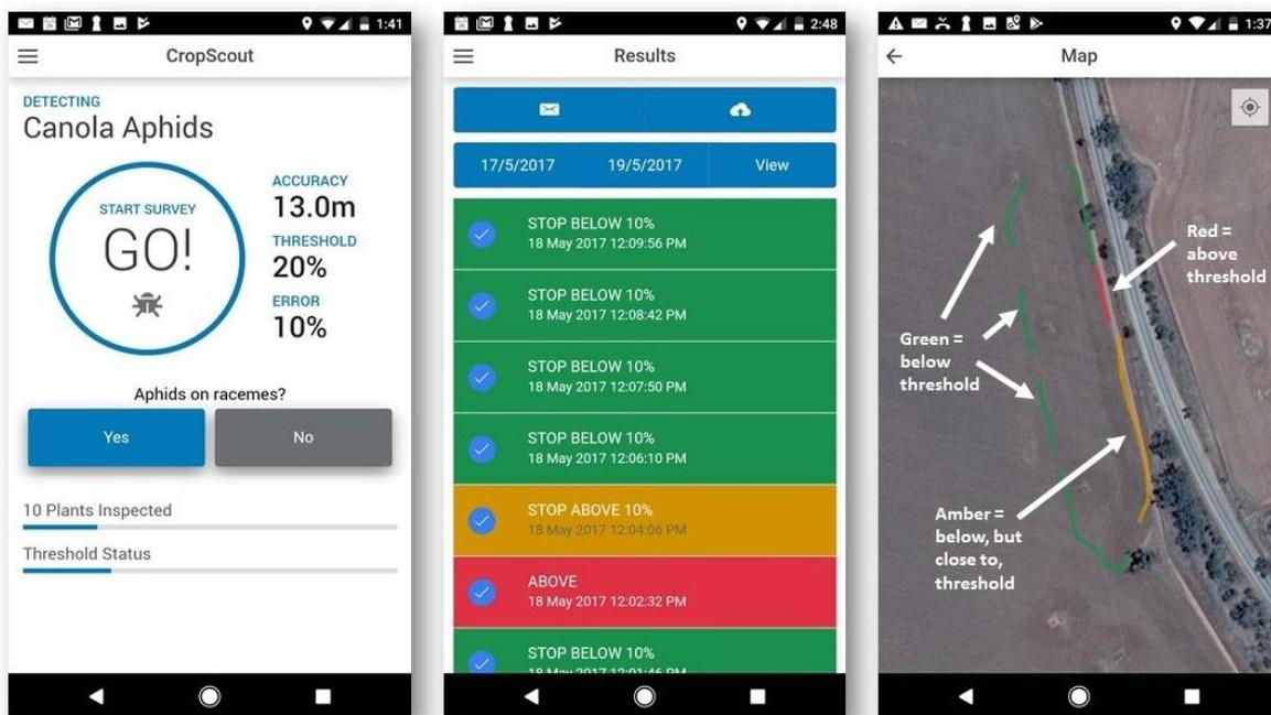
Figure 6. Three mobile phone screen views of the CropScout app showing the sampling interface (left), results list with data export/sync tools (middle) and colour coded maps of spray threshold results (right).
