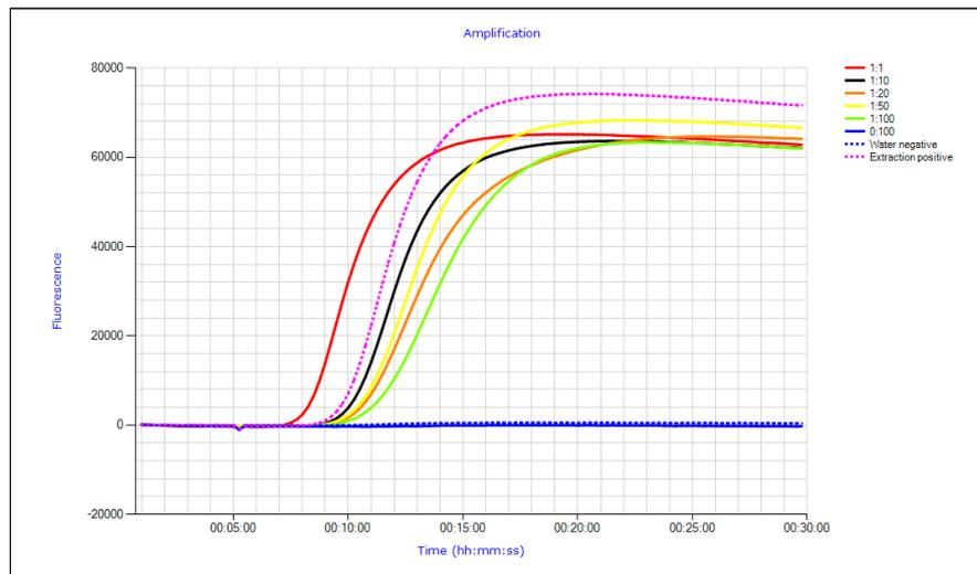
Figure 3. Reverse transcription loop-mediated isothermal amplification (LAMP) of TuYV from serial dilutions of one viruliferous GPA in groups of non-viruliferous GPA.
