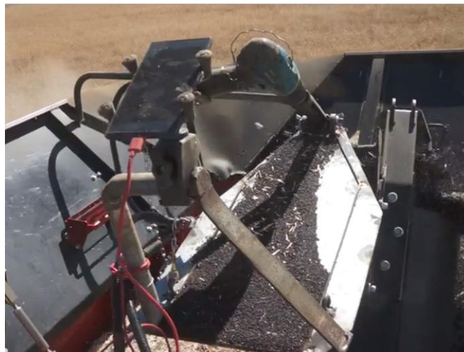
Figure 9. The WheelCam attached to a Case header. Figure 10. The GrainCam attached to the bubble auger.
