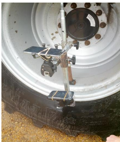
Figure 9. The WheelCam attached to a Case header. Figure 10. The GrainCam attached to the bubble auger.
