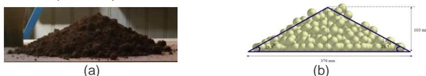
Fig 1. Angle of repose test for calibration (a) Laboratory test, (b) DEM simulations.
