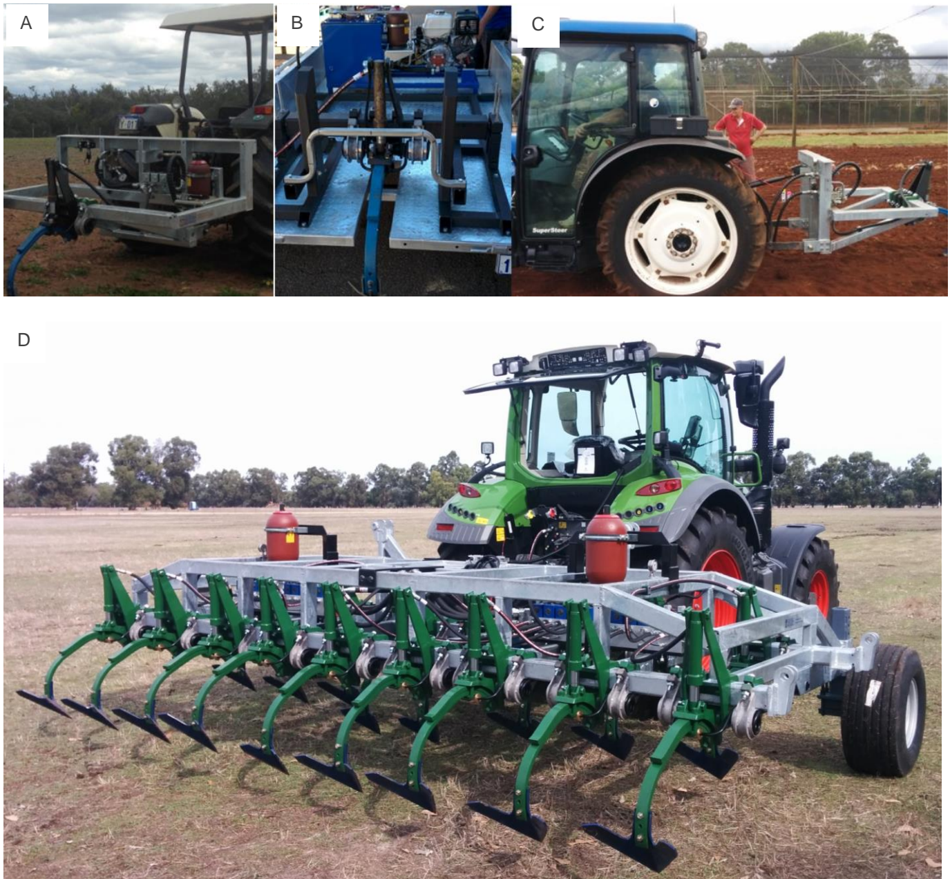
Figure 1. Initial proof-of-concept rig (Shenton Park) (A), Narrabri trailer mounted self-powered rig (B) and QDAF 3-point-linkage rig (C) and Pre-commercial rig – the ‘Weed Chipper’ (D) used in the testing and validation of targeted tillage fallow weed control.
